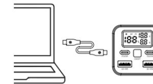
Connect the PowerPort with the USB Type C port using the supplied USB Type C to USB Type C cable to your computer.
